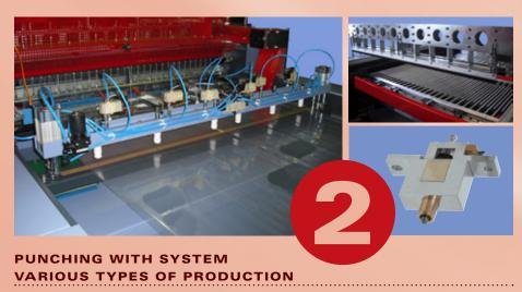
Different products require different production steps. With our variable punching systems we offer versatile custom-tailored production types according to the individual requirements. Our scope of services includes pneumatic and electromagnetic hole punching units, which can produce, depending on the application a package- or single-punch and either punch in cycles or continuously. Whether ventilation or suggestion holes – we punch in versatility with system.
